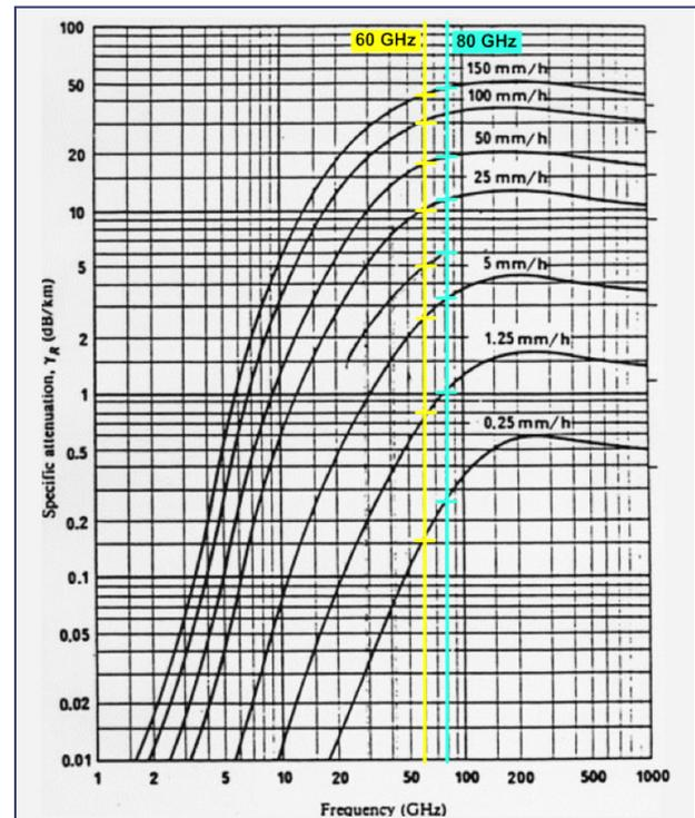
Figure 1. Attenuation due to Rain vs Frequency
