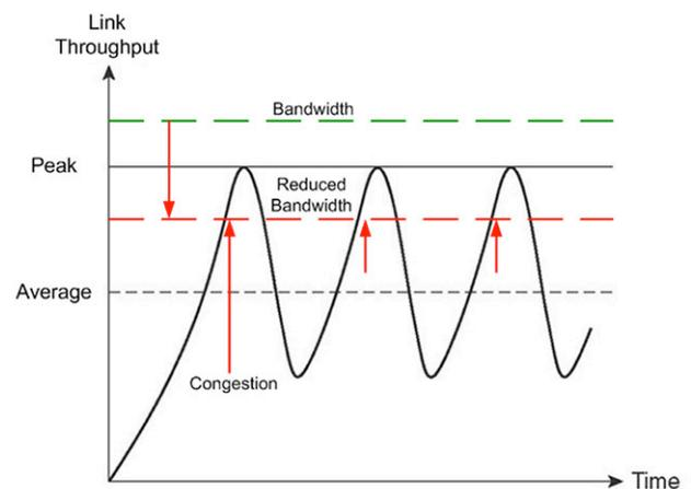
**Figure 2. Impact on Link Throughput from Bandwidth Reduction**
