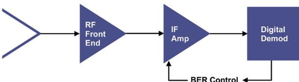
Figure 4. Intelligent AGC with Bit Error Rate Control
