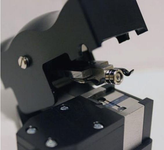
Figure 10. Fiber Optic Coupler for Tapping Without Detection
