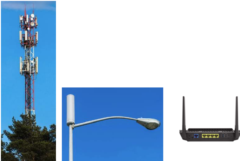
Figure 3. Omnidirectional Antennas: Macrocell, Microcell, and Wi-Fi Router
