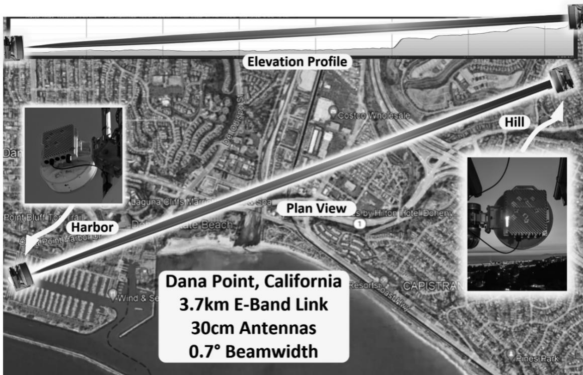
Figure 9. Dana Point E-Band Link, 3.7 km, 10 Gbps Full Duplex with Plan and Elevation Views
