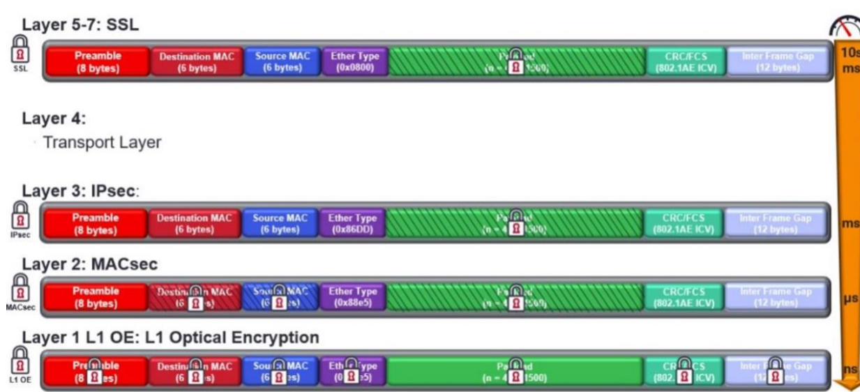
Figure 12. OSI Network Layers Shown with Various Encryption Schemes
